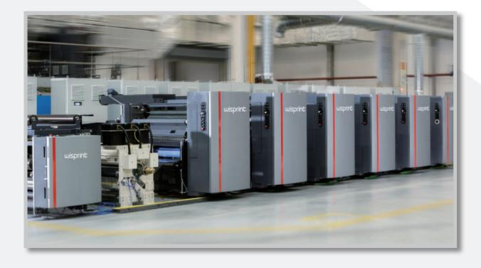
The Litho Vario is a web offset press that allows for variable print repeat lengths. This press was developed for packaging customers to print short production runs and still stay competitive due to the lower cost of web offset consumables. Capable of printing on film, paper or board, the Litho Vario is very versatile for the packaging printer.
